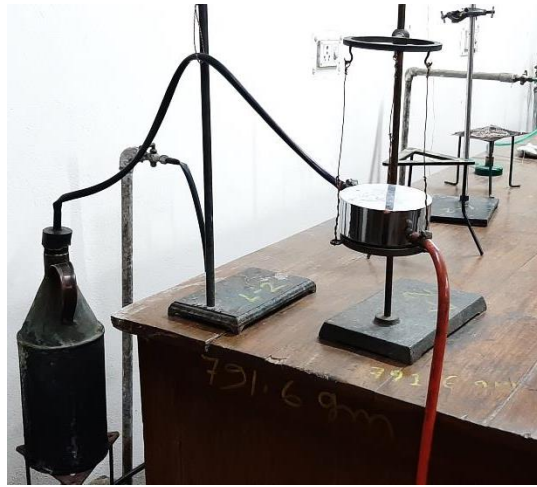
Determination of the thermal conductivity of a bad conductor by Lee's method
