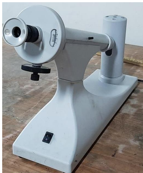
Determination of the specific rotation of sugar solution by a Polarimeter
