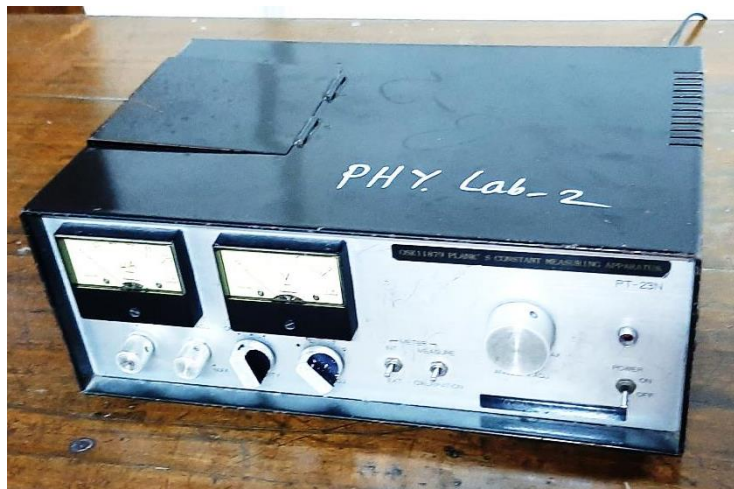
Determination of the threshold frequency for the material of a photocathode
