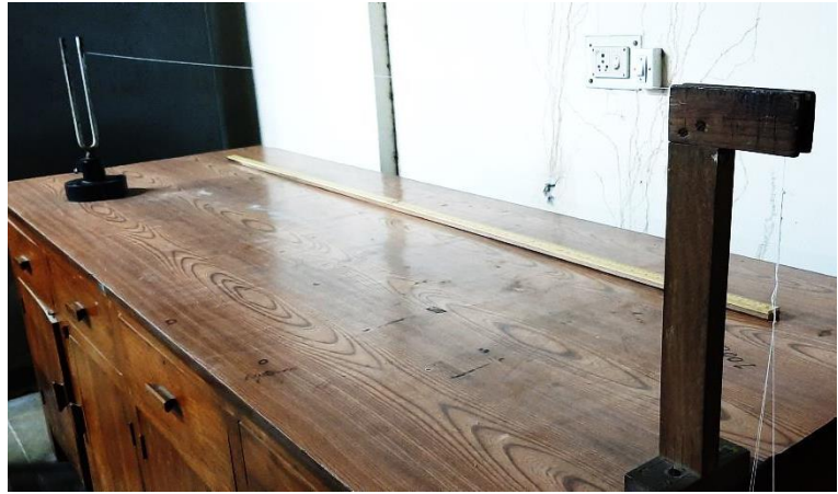
Determination of the frequency of a tuning fork by Melde's apparatus.
