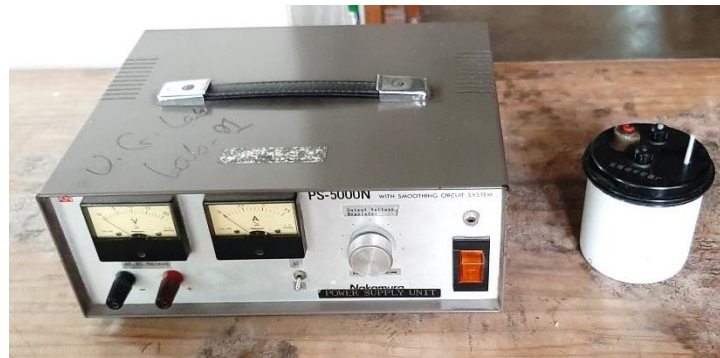
Determination of the mechanical equivalent of heat by the electrical method
