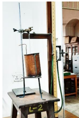
Determination of the pressure-coefficient of air by a constant volume air thermometer
