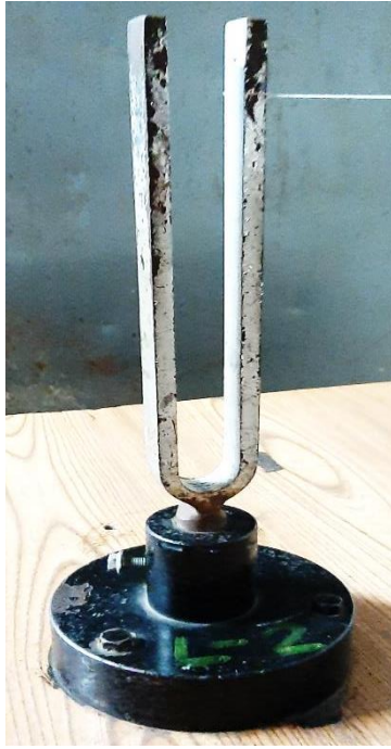
Determination of the frequency of a tuning fork by Melde's apparatus.
